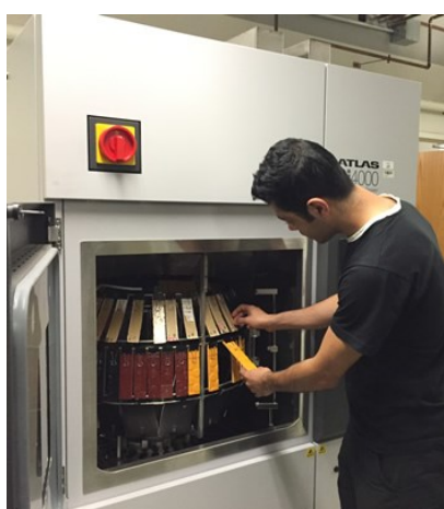
Siavash Vahidi removing polymeric material samples from the weatherometer.
